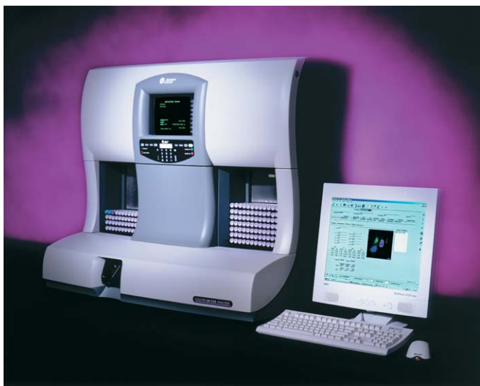
Figure 5. The latest descendant of the Model A Coulter Counter ® , the LH 750 analyzer, is a fully automated instrument that determines 26 reportable hematological parameters. When combined with the LH Slide Maker and the LH Slide Stainer to form the LH 755 Hematology System, it also automates preparation of microscope slides from selected whole-blood samples.
